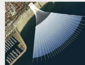
HDD wells (i.e., Neodren)
